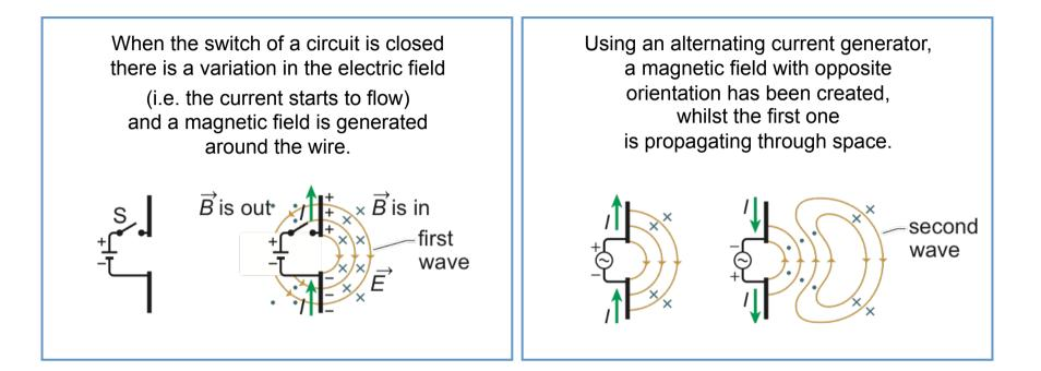
This circuit is an **antenna** that emits electromagnetic waves in all directions.
