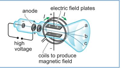
In 1897, Thomson used an apparatus, which made use of electric and magnetic fields, to measure the value of *e/m* (charge/mass) for cathode rays.
