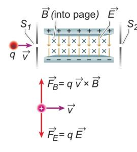
Only particles whose velocities are such that the magnetic and electric forces balance each other will pass through both slits:
