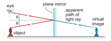
A ray of light from the top of the chess piece reflects from the mirror. To the eye, the ray seems to come from behind the mirror. The bundle of rays from the top of the object appears to originate from the image behind the mirror, which appears reversed, left to right.
