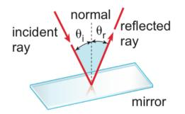
$\theta_i$  is the angle between the incident ray and the normal.  $\theta_r$  is the angle between the reflected ray and the normal.
