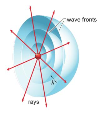
Consider a point source that emits light in all directions. To graphically represent a wave from the source, a spherical surface is drawn through all points on the wave that are in phase (in step with one another). This surface of constant phase is called a **wavefront**.
