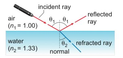
When a ray of light is directed from air into water, part of the light is reflected at the interface and the remainder is refracted into the water, towards the normal.
