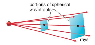
The radial lines pointing outward from the source and perpendicular to the wavefronts are called **rays**. Rays correspond to the direction of flow of radiant energy.
