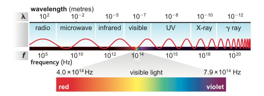
The visible spectrum: only waves with frequencies between about  $4.0 \times 10^{14}$  Hz and  $7.9 \times 10^{14}$  Hz (390 to 750 nm) are perceived by the human eye as visible light.
