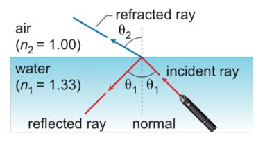
When a ray of light is directed from water into air, the ray that passes into the air is refracted away from the normal.
