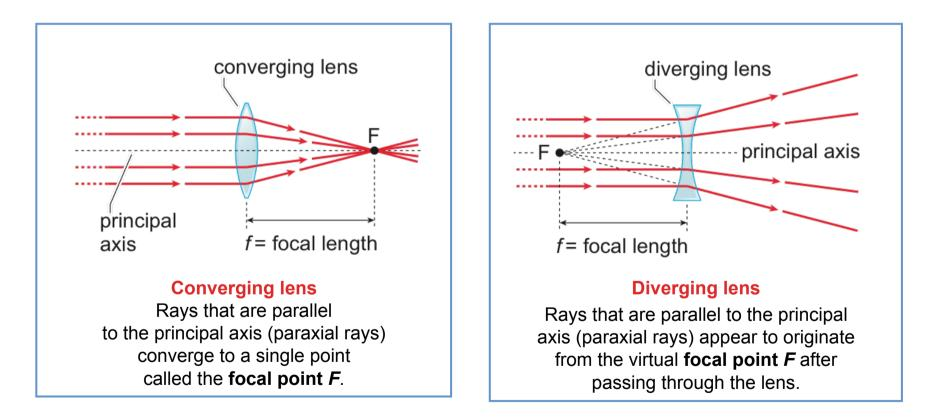
The distance between the focal point and the centre of the lens is the **focal length** *f*.
